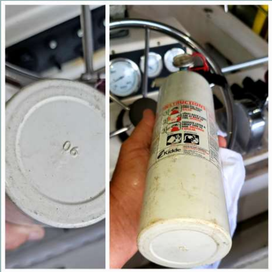
Above is the fire extinguisher that came with my Shamrock17. On close inspection, it appears to be out of date.
