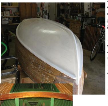
When the boat was turned again, a fillet was added to the top side of the rails with a strip of glass following. After fairing the topsides a layer of fiberglass was applied, followed by two-part primer and paint.
