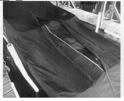
A linear split in the boat cover with closure snaps and Velcro edges will allow the boat to be covered during winter storage for replacement of humidity which prevents plank warping.
